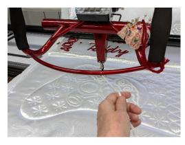
The machine will automatically tie off when the brim is done and pause before moving to the ball of the hat.
