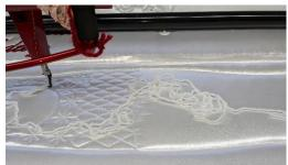
Hold onto the yarn and the thread and click OK. Let it do the tie off and drop the speed down to 2 (20%).
